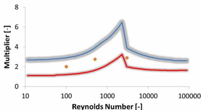
Fig. 8: Shear stress multiplier when using hiTRAN inserts. Bottom line (Red) low dense insert. Top line (blue) high dense insert, yellow points data from LDV experiments
