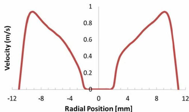
Fig. 9: Velocity profile with CFD simulation, Reynolds 1000
