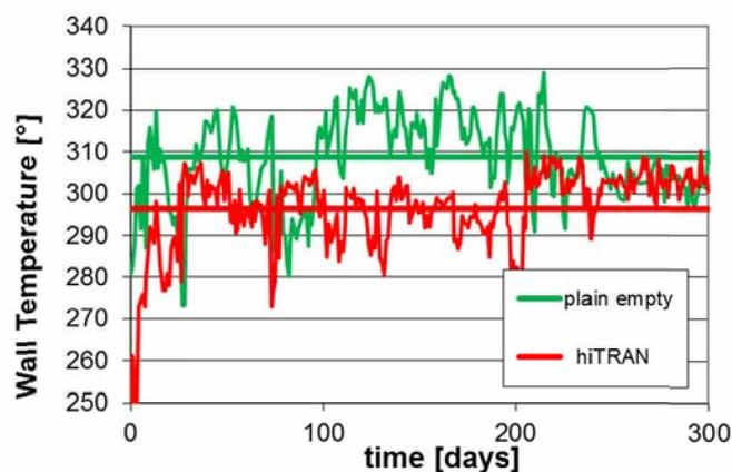
Fig.15: Tube wall temperatures before and after installation of hiTRAN
