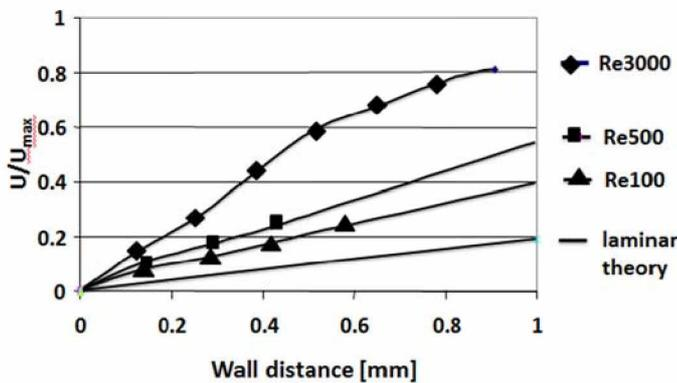
Fig. 5.: Near wall velocity profile for different Reynolds numbers compared to plain empty tube theory for a constant insert geometry
