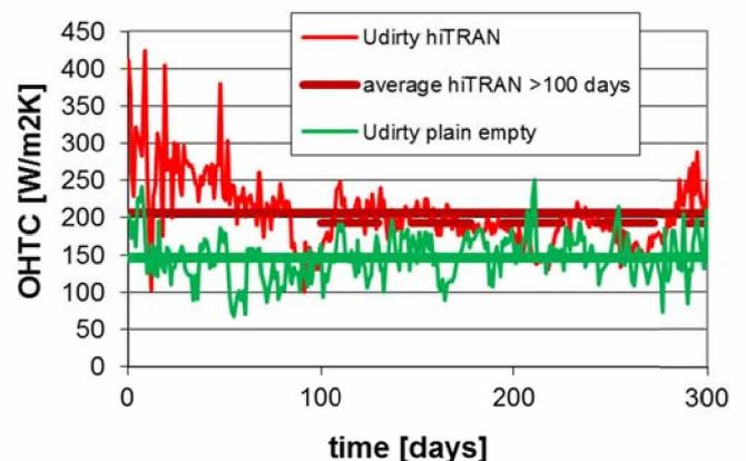
Fig. 14: Overall heat transfer coefficient over time for plain empty tube and hiTRAN System
