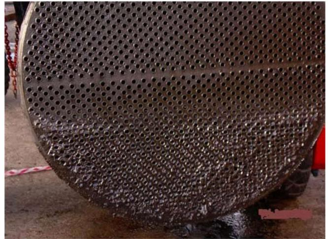
Fig. 13: Investigation of fouled AES VDU / Feed heat exchanger.
