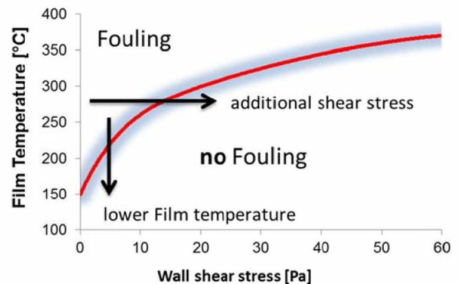
Fig. 1: Threshold model and implication of additional shear stress and lower film (wall) temperatures.
