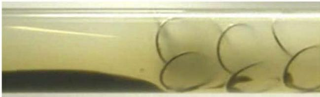
Fig. 12: Water flow suspension. Average particle size 50 $\mu$ m, density 2420kg/m<sup>3</sup>
