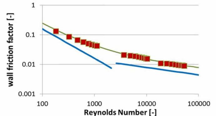
Fig. 7: Measured wall fanning friction factor for a particular hiTRAN geometry compared with plain empty tube data as function of Reynolds number
