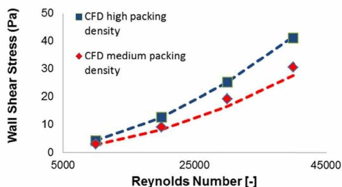
Fig. 10: Wall shear stress correlations from measured data for medium dense (red dashed line) and high dense (blue dashed line) hiTRAN inserts with CFD simulations
