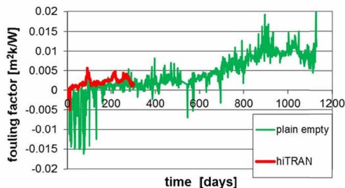
Fig. 16: Fouling factor for plain empty tube and hiTRAN operation
