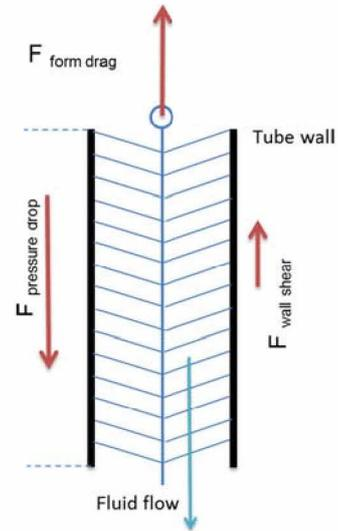
Fig.6: Measurement principle to determine the increased wall shear force created with the addition of hiTRAN insert
