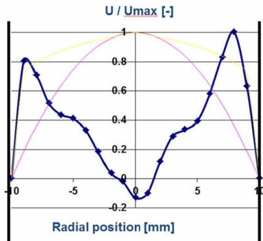
Fig. 4: Normalized velocity profile at Reynolds Number 500 just after hiTRAN insert. For plain tube comparison Yellow line - turbulent profile, pink line -laminar profile are shown
