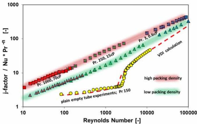
Fig. 3: Typical heat transfer performance of two hiTRAN geometries.
