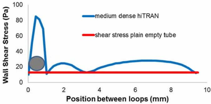
Fig. 11: Shear stress distribution between adjacent hiTRAN loops. Water, flow velocity 2.06m/sec Reynolds number 30000
